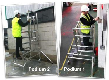
Please Note: Stepfold Podium 1 is assembled in the same way as Stepfold Podium 2, with just 1 less horizontal brace.
